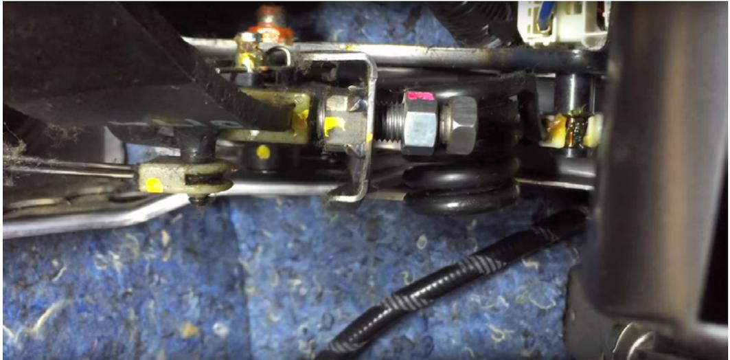
2. Ensure that the locking nut is tightened back against the bracket to avoid unwanted adjustment when the clutch pedal is used.
