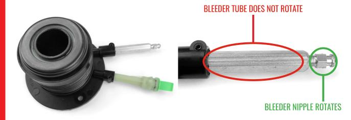
It is recommended to loosen the bleed nipple initially before installing the CSC so that a second ring spanner can be used to support the hex tube and avoid excess force being applied to the CSC body.
