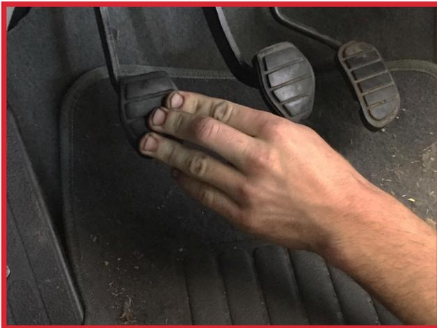
Fill the reservoir with fluid and allow the fluid to gravity bleed. Once fluid is flowing, use your hand to slowly depress the pedal by 3/4 stroke and back checking the reservoir level. Continue until no more air bubbles are flowing.
