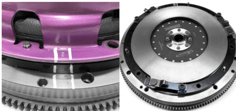
2. Remove the intermediate plate from the flywheel by using a flat blade screwdriver under the cutout sections at the dowels. The bottom disc can now be removed. **Do not lever under the intermediate plate straps or loosen the bolts holding the straps on the intermediate plate.**
