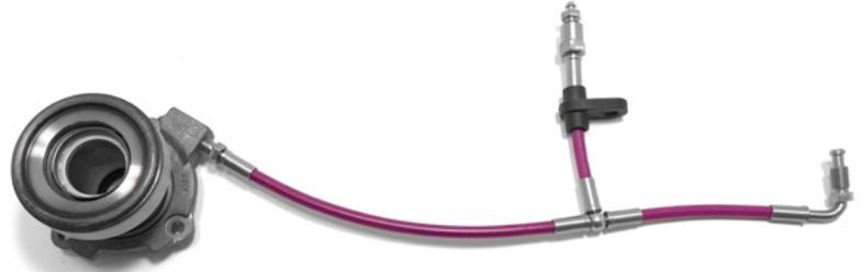
1. Unbolt and remove the original CSC. Thoroughly clean the mounting surface to ensure there are no burrs or debris where the new CSC will mount.
