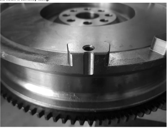
If the flywheel was not indexed before being removed, rotate the engine to Top Dead Centre (align the crankshaft pulley notch with the mark on the timing case). The notch on the flywheel will face down (6 o'clock) when the engine is at TDC.
