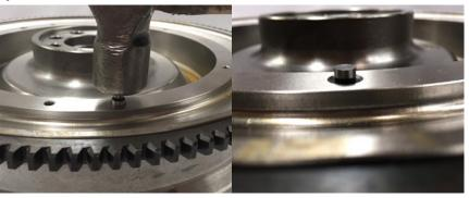
With the dowels in the flywheel, the trigger wheel can be mounted on the dowels. There is only one orientation in which it can fit. Use thread retaining compound on the original M6 bolts and torque them up to 12Nm/9ft.lbs.
