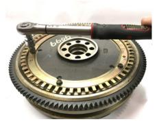
Install the flywheel onto the engine ensuring that the notch in the new flywheel lines up with the mark/ direction you noted when removing the old flywheel. Or if you set the engine to TDC, ensure the flywheel goes on with the notch facing down.
