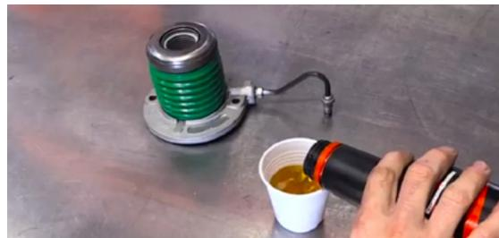
2. Submerge the end of the CSC line into the fluid.
