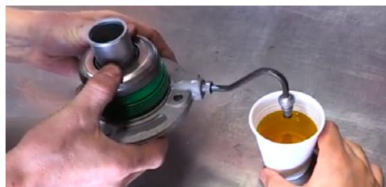
3. Hold the CSC with the fluid port as upright as possible and slowly operate the CSC several times, moving the release bearing up and down. This will induce fluid into the piston.
