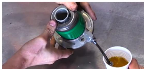
4. After the gearbox has been installed, fill the master cylinder with fresh brake fluid, correct to the vehicle manufacturers specifications. Slowly operate the clutch pedal to induce fluid flow from the master cylinder to the CSC. Note that this process may take up to 50 pedal cycles to appropriately bleed the system.
