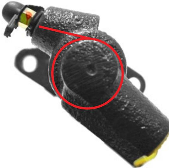
Rotate slave 90° counter-clockwise to ensure air can escape the slave.
