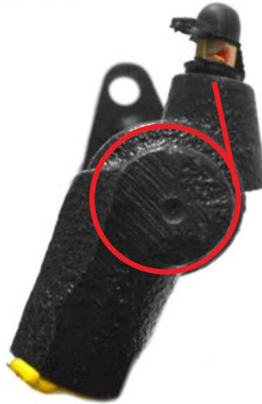
Mounted Position: Air remains trapped in the top of the bore.
