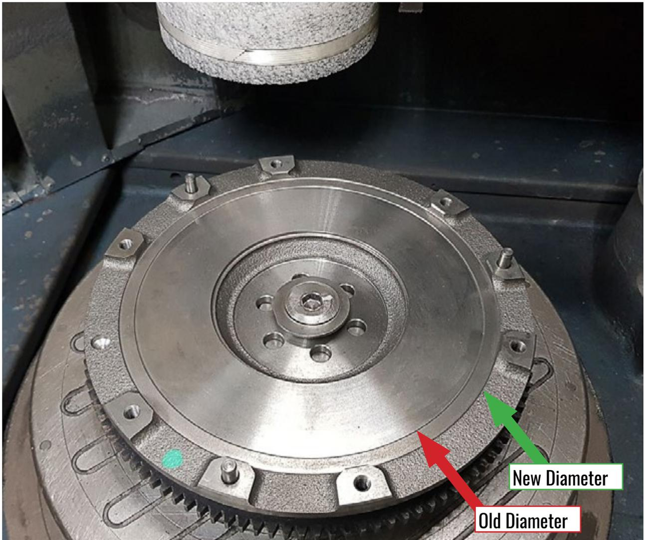
Failure to do so will affect the performance and life of the clutch.
