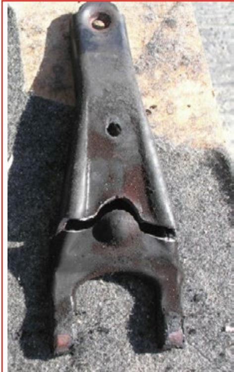
Clutch forks can fracture after excessive wear. It is important to check all points of contact when inspecting them.
