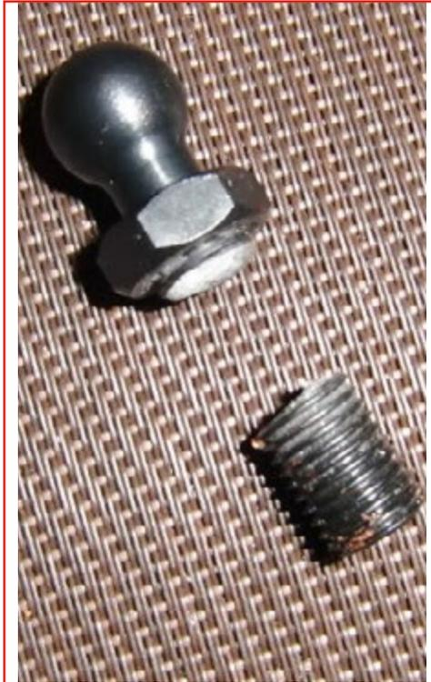
Pivot Balls can wear down in height, or even completely shear like in the above photo. Check for any witness marks of wear
