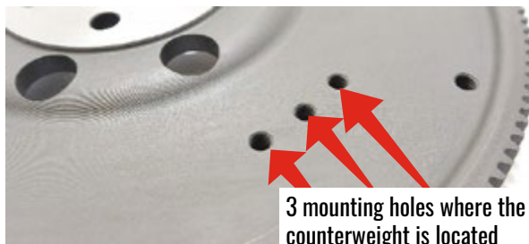
Using a thread locking compound fit the 3 counter sunk headed bolts (as supplied) and torque to 35Nm
