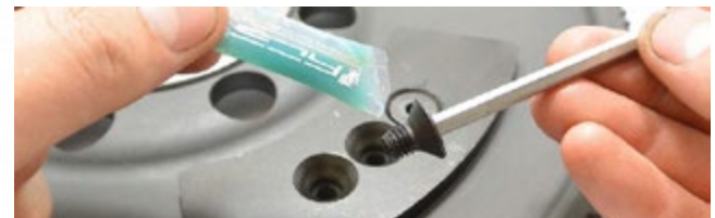
Using a thread locking compound fit the 3 counter sunk headed bolts (as supplied) and torque to 35Nm
