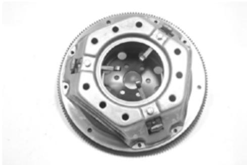
The original lever and spring clutch (CFD28101) has 6 mounting holes which are located either side of the clutch lever.
