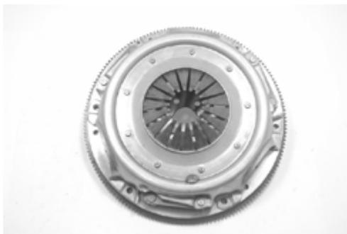
This clutch cover (CFD28102) suits the multi drilled Ford flywheel. The Ford multi drilled flywheel has been designed and drilled to suit various Ford cover stampings. If this cover is used on the Ford single drilled flywheel only 3 mounting holes will locate the cover and the other 3 will need to be drilled and tapped.
