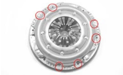
The diaphragm conversion cover (CFD28103) uses the holes marked. This cover suits the single drill flywheel. The clutch cover whilst has 9 bolts holes only 6 are use (3 mounting holes -smaller diameter- and 3 clamping holes-larger diameter) if required the extra holes can be used but the flywheel will need the holes drilled and tapped.
