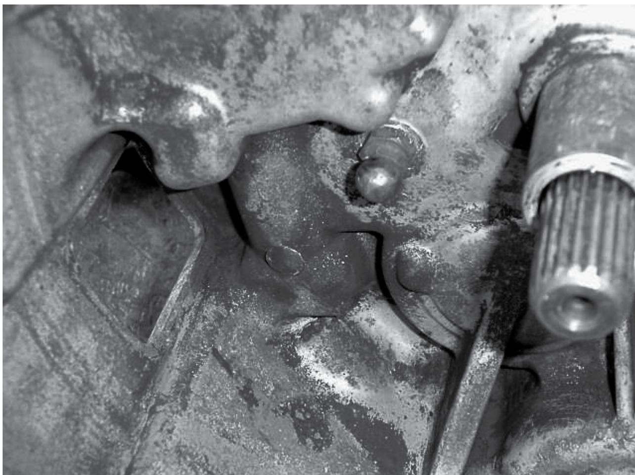
2. Clean bell housing and all other gearbox components. After removal of gearbox, clean all components. Check gearbox bearing nose cone for wear. If worn, it must be replaced to avoid pedal graunch and notchy feel when new clutch is installed.
