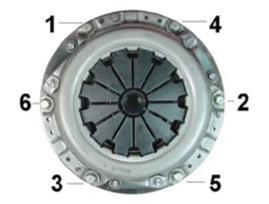
The bolts need to be tightened in a "star" type formation. See picture. Please refer to manufacturers workshop manual for recommended torques.
