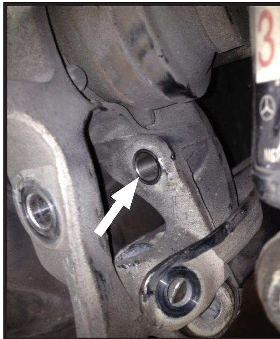
14. REINSTALL AND TIGHTEN THE LOWER CONTROL ARM BOLT. (FIGURES 69, 70)
