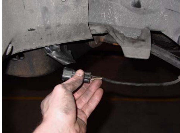
8. Unplug the strut damper solenoid. ↑
