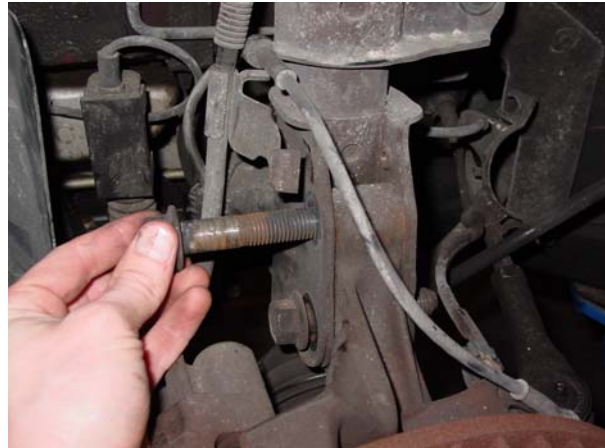
10. Remove the two strut-to-knuckle bolts. ↑
