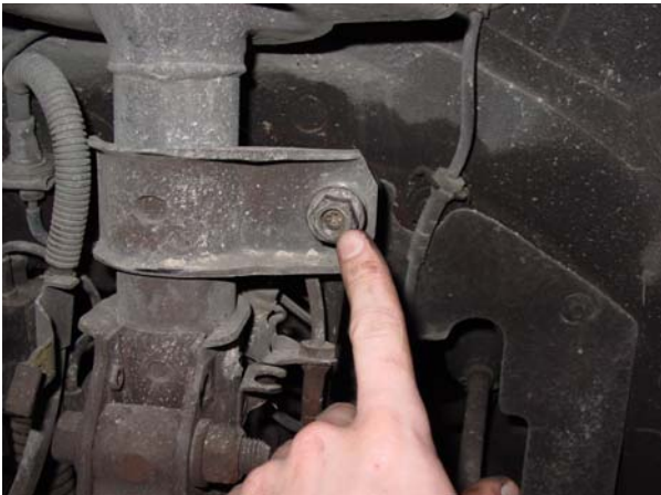
5. Remove nut from stabilizer link ↑
