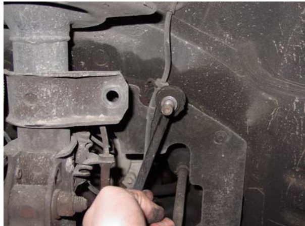
6. Remove stabilizer link from strut. ↑
