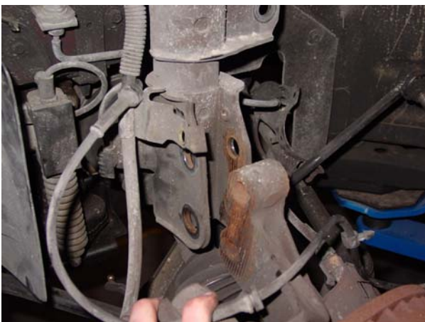
11. Knuckle will fall away from strut. ↑
