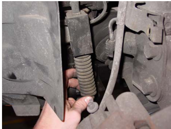
4. Remove the position sensor from upper and lower ball studs. ↑
